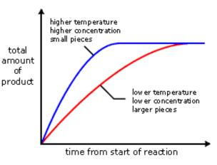
The reaction stops when one of the reactants (the limiting factor) gets used up and the graph goes flat.
