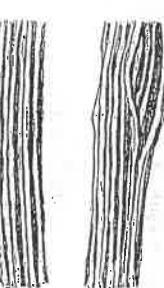
Viscose fibres as seen under a microscope
