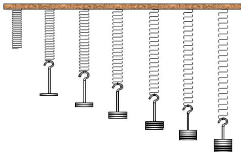
The extension of a spring is directly **proportional** to the force on it. This is called **Hooke's Law**. The greater the force pulling down, the greater the extension of the spring.
