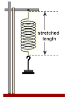
**Elastic** materials will stretch with a force and then return to their original shape when the force is taken away. Springs are elastic.
